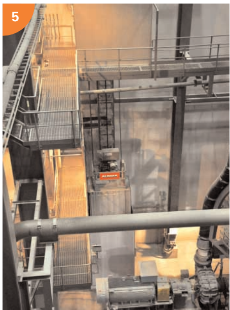
Flotation Elevator: ALIMAK SE 1000 FC Capacity: 1000 kg Lifting height: 20 m
